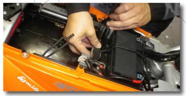
Now attach the unit's cable to the vehicle's battery and fix it in place with cable ties. Make sure the cable won't get damaged by the seat, parts of the casing, or other things. Screw the two poles of the sable to the battery.
