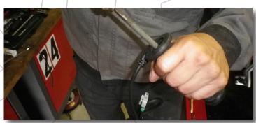
Now, apply some glue to the inside of the grips (two-component glue). The glue should be applied carefully but thoroughly. It also serves as a lubricant and prevents the grips from coming lose after bonding.
