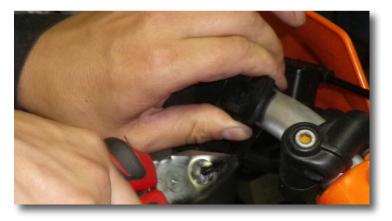
Carefully cut away the excessive belt, without damaging the last (holding) grid on the underside. Leave about 2~3mm of the belt behind the holding grid intact, so the grid has some flexibility and won't accidentally open. If it happens, you will need a new holder!
